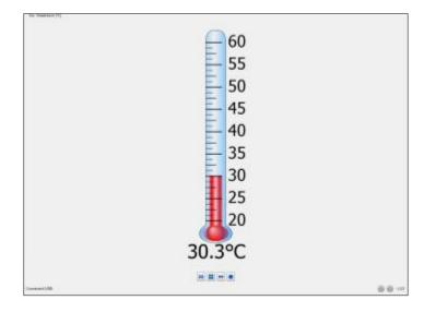
Changing the range of the meter, or the type of sensors displayed by the meter is done with a right click on the sensor name located at the top left corner of the meter. The right click opens a dialog box where the sensor type and new range can be changed.
